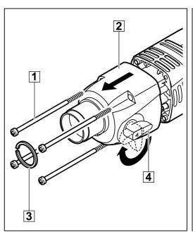
Removing the switch lever
