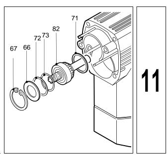
Removing the motor cover
