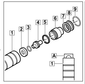
Assembling the spindle (mounting the inner parts)
